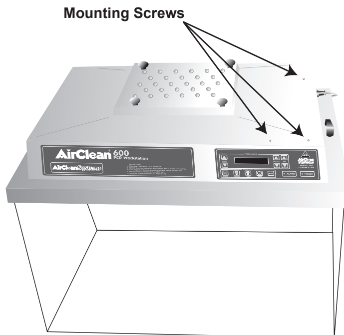
Figure 9, Removing the UVTest™ Controller from the AC632 model.
