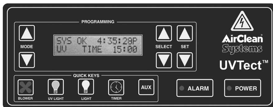
Figure 6, Control panel layout.
